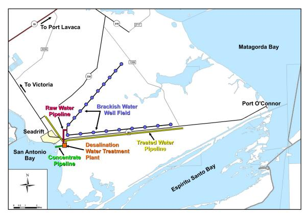
Figure ES-1. Southern Calhoun County Brackish Groundwater Desalination Project
