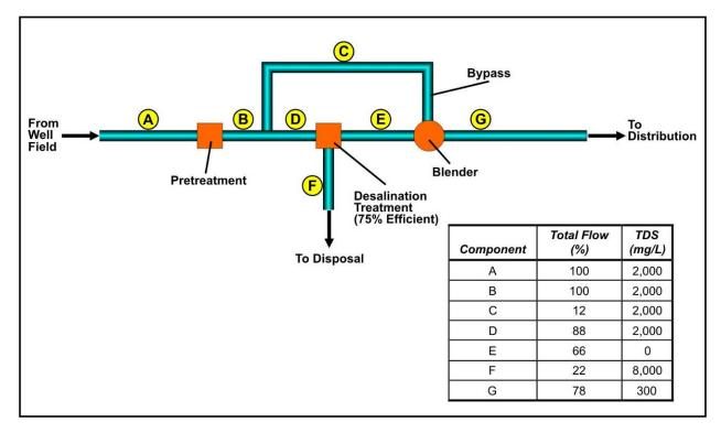
Figure 2-2. Flow Diagram for a Desalination Water Treatment Plant
